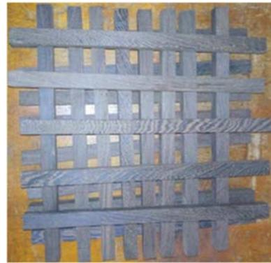
Figure 2. WW specimens of  $360\times 20\times 20\text{ mm}^3$ .
