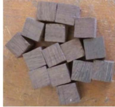
Figure 1. WW specimens of  $20\times 20\times 20\text{ mm}^3$ .
