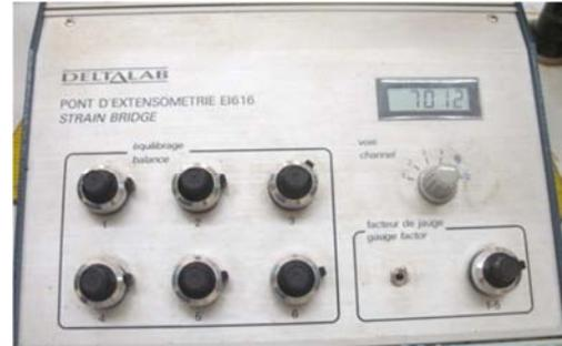
Figure 6. Numerical strain bridge.
